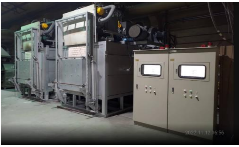
建置蓄熱式燒結爐
